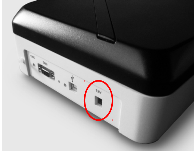
Power Supply Connection.
