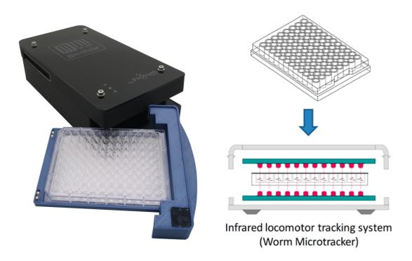
As the animals cross the sensor grid, locomotor activity is detected as interruptions in light beams;
