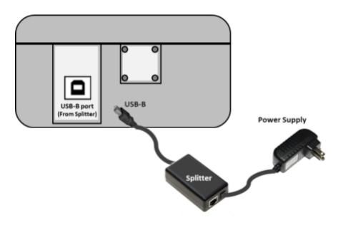
2. When you connect the Power Supply to the green light on top of it should turn on and the red light will flash (While the system is being checked).
