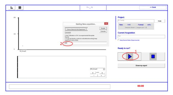
3. The software will automatically calibrate the 96 sensors into the system to recognize the worm movement. This calibration will take about 1 minute for the first time, and a few seconds in the future.
