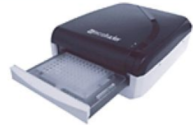
(C) Record the activity of the plate with worms using WMicrotracker ONE
